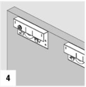
Mount the upper roller for inner doors keeping the adjusting screw facing toward the edges of door.
