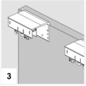
Mount the upper roller to outer doors, keeping the adjusting screw facing toward the edges of the door.
