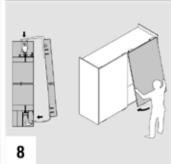
Mount the outer door on the upper track. Swing the lower part of door onto guide rail, push until guide rollers click into position.
