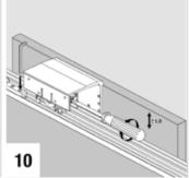
Move softclosers to create position and lock with allen key. Adust height and plumb of door using screwdriver in the adjusting screws in upper.
