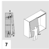
Mount the inner door on the upper track. Swing the lower part of door onto guide rail, push until guide rollers click into position.
