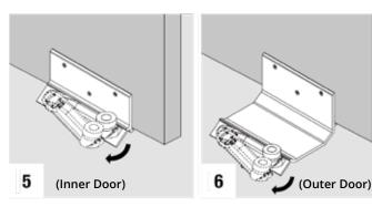
Mount the lower guides with the wheel towards the edge of the door. Prior to fitting open arms by rotating them outward.
