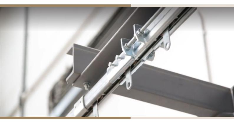
The Multirail™ Auto is ideal for any application needing an automated conveyor system. Multirail Auto comes with a continuous trolley and chain loop and multiple hanging eyes make it easy for the operator to load product to the line. A drive unit powers the chain around the heavy duty track.
