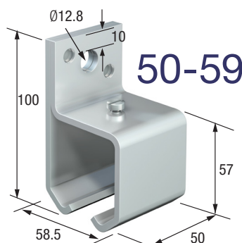
50-59 Wall fixing steel bracket for the upper track.
