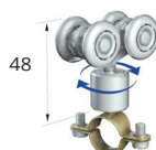
Double rotating axle wheel hanger with pipe clamp, 25kg capacity Code: 16mm Pipe clamp: 20-1224-016 26mm Pipe clamp: 20-1224-026 32mm Pipe clamp: 20-1224-032
